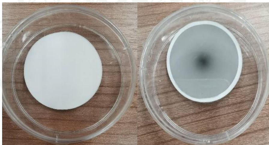
Figure 97 MCE filter (Left: cold test's filter and Right: hot test's filter) from passenger car
