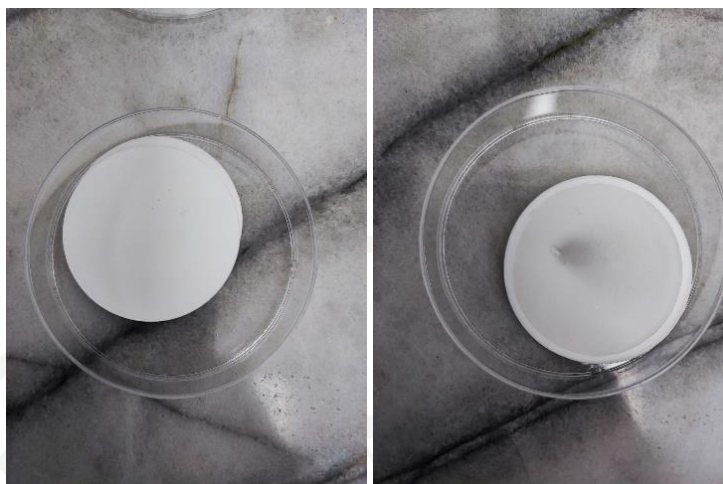
Figure 104 MCE filter (Left: cold test's filter and Right: hot test's filter) from SUV
