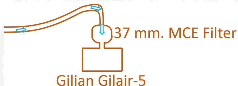
Figure 35 Schematic Diagram of Gilian Gilair-5 Air Sampling Pumps with MCE filter paper
